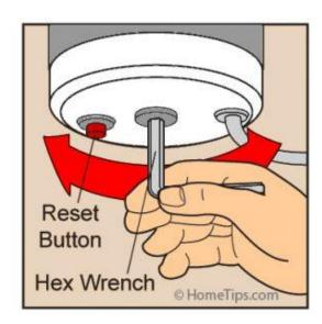
**3.** To clear a jam, insert a 1/4-inch <u>hex wrench</u> into the hex-shaped hole in the underside of the garbage disposal and crank both directions a few times to free-up the impellers.
